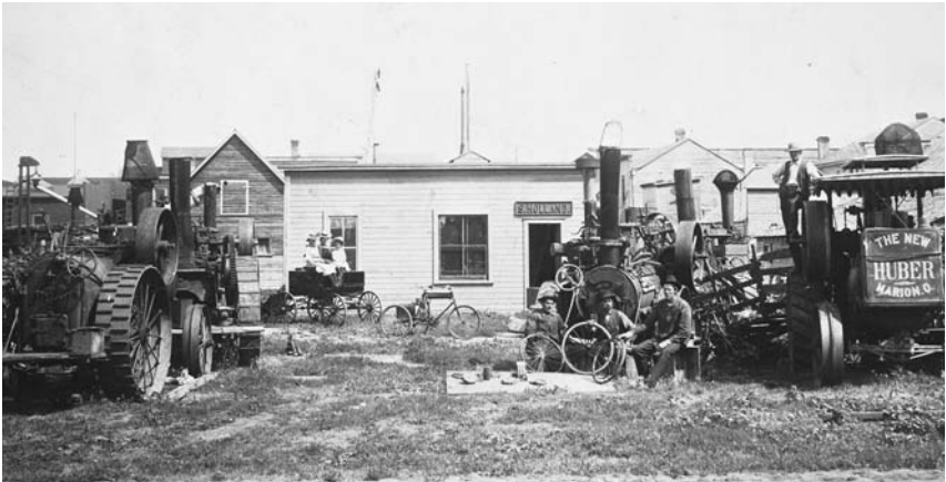
Fig. 8. Samuel Holland's Blacksmith Shop in Park River, N.Dak., ca. 1910, showing the diversity of equipment blacksmiths might be called on to repair in rural communities. To the far left and right sit steam tractors. In the foreground three men hold wire bicycle-style wheels with pneumatic tires. In the center middle ground sits a three-wheeled motorcycle, and behind it are three women sitting atop a horseless carriage. Courtesy of Fred Hulstrand History in Pictures Collection, North Dakota Institute for Regional Studies, North Dakota State University, Fargo.
