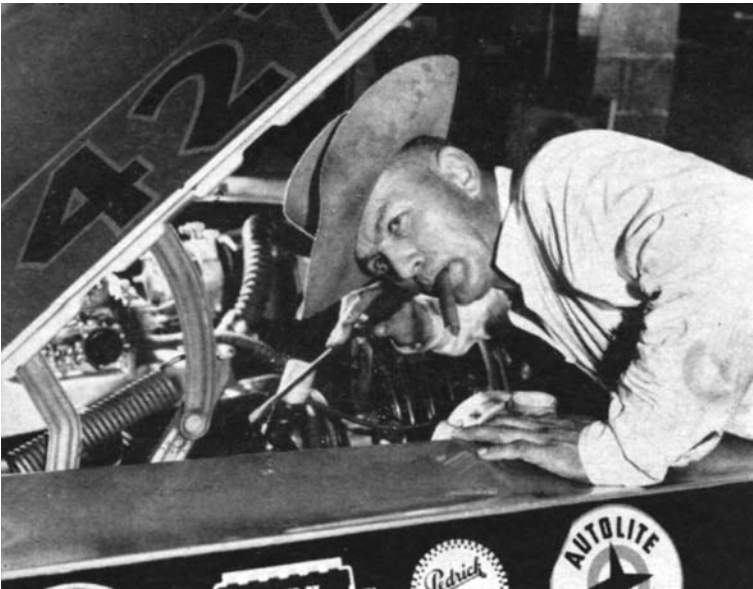
Fig. 24. Smokey Yunick using a screwdriver as a sounding rod to listen to a race engine. Reprinted from Popular Science , January 1964, 94.
