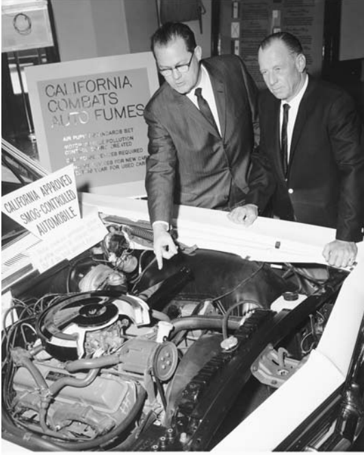
Fig. 27. Automobile Club of Southern California executive vice president, Joe Havenner (left), points to belt-driven compressor of emission control system on a 1966 Chevrolet. Hoses leading over valve covers, down toward exhaust manifolds, carry additional oxygen to exhaust stream. Photo courtesy of Automobile Club of Southern California Archives.
